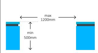
The minimum height for vertical fixed structure is 500 mm. An increased height of 900 mm will make the measures more conspicuous
