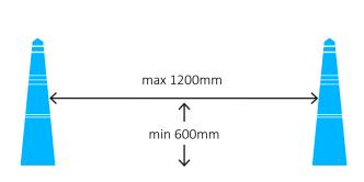
The maximum clear distance between adjacent VSB must be no greater than 1200mm, this distance must be measured between structural elements at a height of 600mm above ground level.
