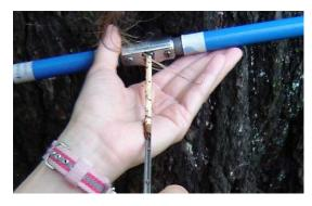
**RESISTOGRAPH -** This measures the drilling resistance of a needle drill. Data can be displayed as a paper trace (shown opposite) or as a digital output for a more detailed assessment of the internal condition of the tree.
